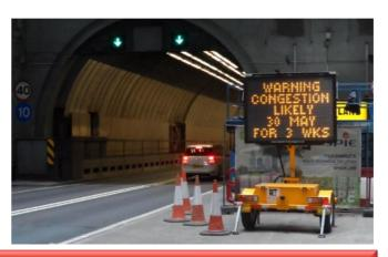
The VMS-M can be programmed locally by the onboard touchscreen or by the web based app remotely. The amber LED Display can be used to display MS4 style pictograms or up to 5 lines of text. It can be used in conjunction with additional hardware such as radar, data logging and queue detection to offer a fully scalable I.T.S solutions such as Journey Time Measurement.
