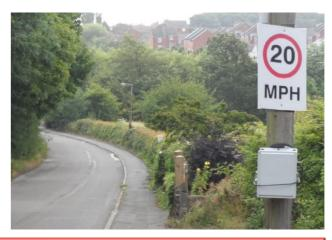
The Speed Spy roadside data recorder is a covert data collection tool to produce traffic reports for analysis. Used by local authorities and comminty speed watch groups, it gives an accurate view of traffic speeds and flow. Housed within the enclosure is a 12v rechargeable battery which can power the Speed Spy for up to 4 days. The Speed Spy comes complete with a fixing kit to mount it to any lamppost at the roadside.
