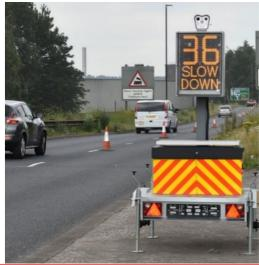
The SDT-VAS Vehicle Activated Sign is a compact trailer designed to slow traffic entering temporary traffic management or construction sites. The SDT-VAS has an onboard battery bank with solar charging capabilities to offer autonomous operation all year round. If viewing traffic flow is important on site, the SDT-VAS can have a camera fitted which can stream live footage in real time to any smartphone via a bespoke app.
