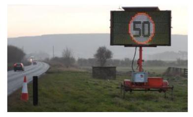
The VMS-5C can be programmed locally by the onboard computer or by the web based app remotely. The 5 colour LED Display can be used to display MS4 style pictograms or up to 5 lines of text. It can be used in conjunction with additional hardware such as radar, data logging and queue detection to offer a fully scalable I.T.S solutions such as Journey Time Measurement.
