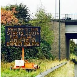
The VMS-4 can be programmed locally by the onboard computer or by the web based app remotely. The amber LED Display can be used to display MS4 style pictograms or up to 5 lines of text. It can be used in conjunction with additional hardware such as radar, data logging and queue detection to offer a fully scalable I.T.S solutions such as Journey Time Measurement.
